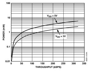
Figure 32. Power vs. Throughput Rate for Power-Down Mode
