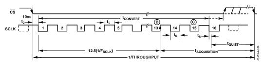
Figure 28. Serial Interface Timing Example
