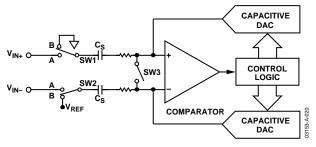
Figure 20. ADC Conversion Phase
