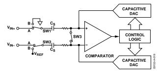
Figure 19. ADC Acquisition Phase
