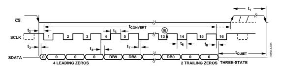
Figure 3. AD7441 Serial Interface Timing Diagram
