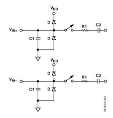
Figure 24. Equivalent Analog Input Circuit; Conversion Phase—Switches Open; Track Phase—Switches Closed When no amplifier is used to drive the analog input, the source impedance should be limited to low values. The maximum source impedance depends on the amount of total harmonic distortion (THD) that can be tolerated. The THD increases as the source impedance increases and performance degrades. Figure 25 shows a graph of THD versus analog input signal frequency for different source impedances.
