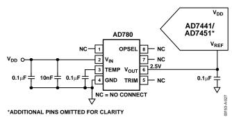
Figure 27. Typical  $V_{REF}$  Connection Diagram for  $V_{DD} = 5 V$
