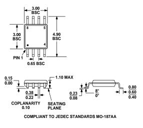
Figure 37. 8-Lead Mini Small Outline Package [MSOP] (RM-8) Dimensions shown in millimeters
