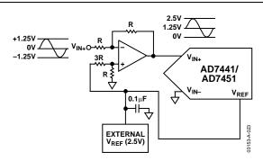
Figure 23. Op Amp Configuration to Level-Shift a Bipolar Input Signal
