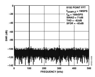
Figure 9. AD7451 Dynamic Performance for  $V_{DD} = 5 V$
