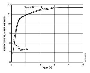
Figure 15. ENOB vs.  $V_{REF}$  for  $V_{DD} = 5 V$  and 3V
