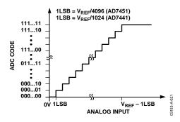
Figure 21. AD7441/AD7451 Ideal Transfer Characteristic
