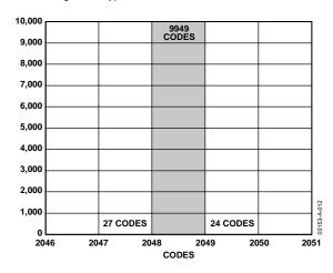
Figure 12. Histogram of 10,000 Conversions of a DC Input for the AD7451
