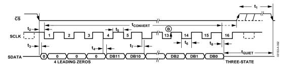
Figure 2. AD7451 Serial Interface Timing Diagram
