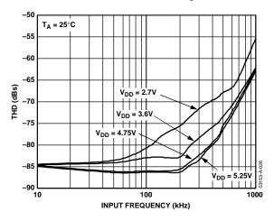
Figure 26. THD vs. Analog Input Frequency for Various Supply Voltages
